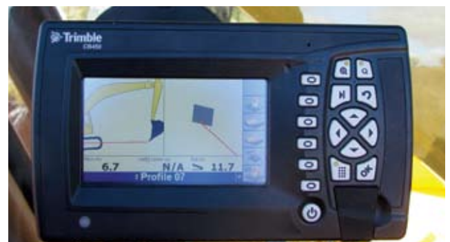
Designed for use in harsh construction environments, the Trimble CB450 Control Box brings an enhanced user experience to the excavator operator and makes it easier to achieve the desired depth and slope with less fatigue and reduced rework
