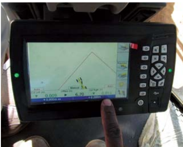
The new state-of-the-art Trimble CB460 Control Box greatly enhances the operator experience on all GCS900 equipped machine types with more power, more memory, and a large seven-inch screen display of 3D profile information, grade guidance, and warnings. As the premium display in the GCS900 portfolio, it can be configured for operation in 2D or 3D mode based on the requirements of the contractor
