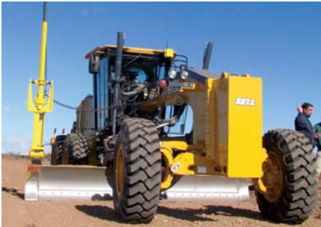
The automatic control of the blade with Trimble GCS900 with Universal Total Station or with Laser augmentation maximises motor grader performance. Whether grading simple pads and slopes or complex design surfaces and alignments the operator can get to grade at high speeds, without sacrificing grade control accuracy or quality of the final graded surface
